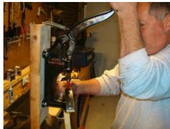
This is a process which requires three sets of hands but in a Model T only two sets can fit. After getting them out, the old material was stripped, new material was riveted on, and then the process of getting them back in be-
